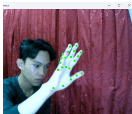
Figure 7. The cursor follows a landmark or point on the fingertip
